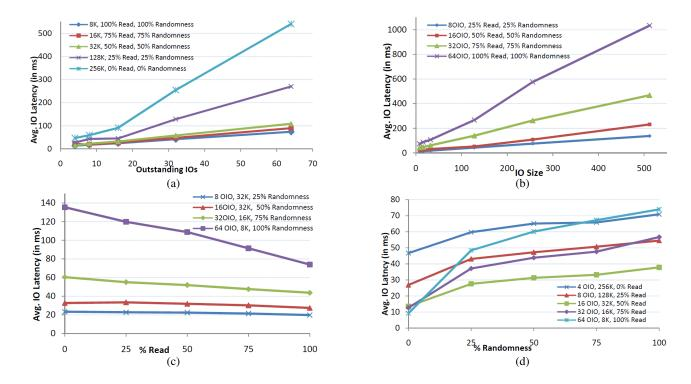
Figure 4: Variation of IO latency with respect to each of the four workload characteristics: outstanding IOs, IO size, % Reads and % Randomness.
