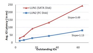
Figure 8: Device Modeling: different disk types
