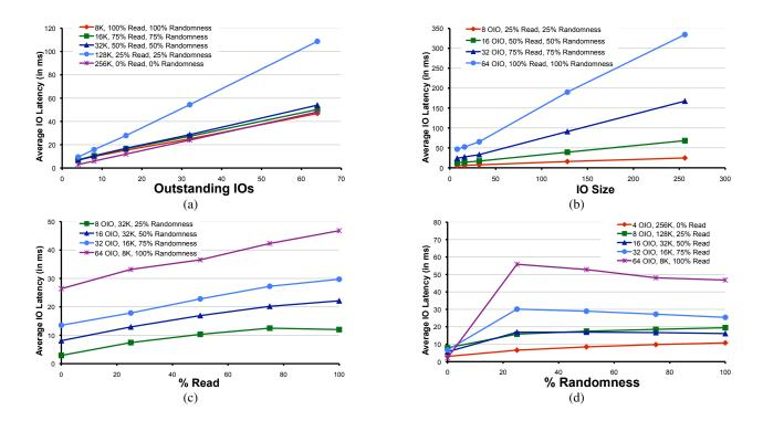
Figure 2: Variation of IO latency with respect to each of the four workload characteristics: outstanding IOs, IO size, % Reads and % Randomness.
